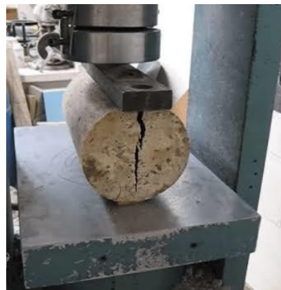
Figure 2.3: Split tensile strength test setup for cylinders.
