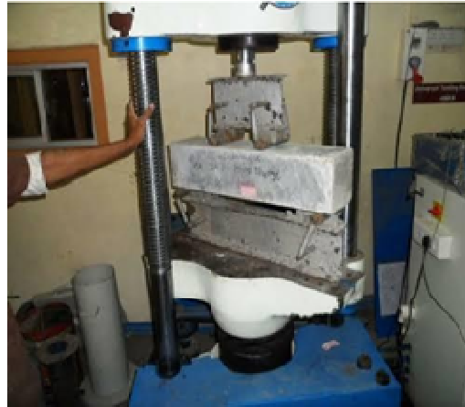
Figure 2.4: Flexural strength test setup for prism
