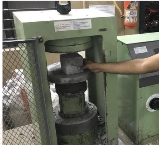
Figure 2.2: compressive strength test setup for cubes
