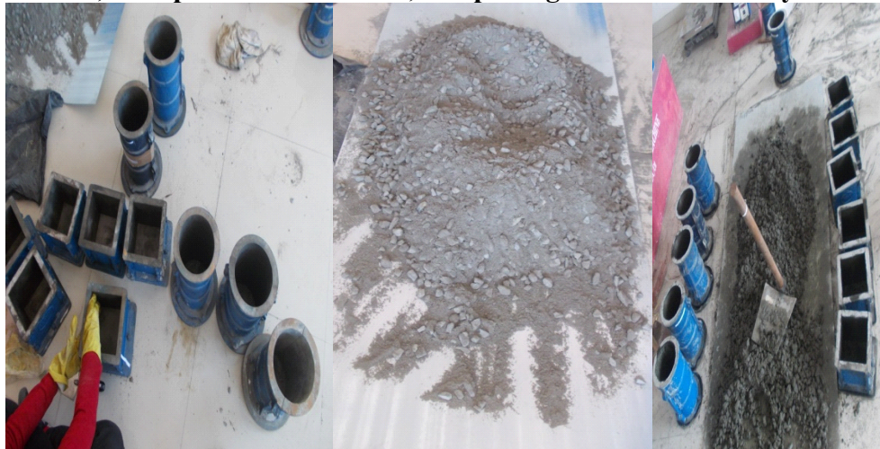
(A) Oiling of Cubes & Cylinder (B) Dry mixing (C) Filling of Moulds
