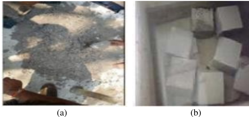
Figure 4: (a) Mixing of concrete and (b) Curing of Cube at Standard temperature in water
