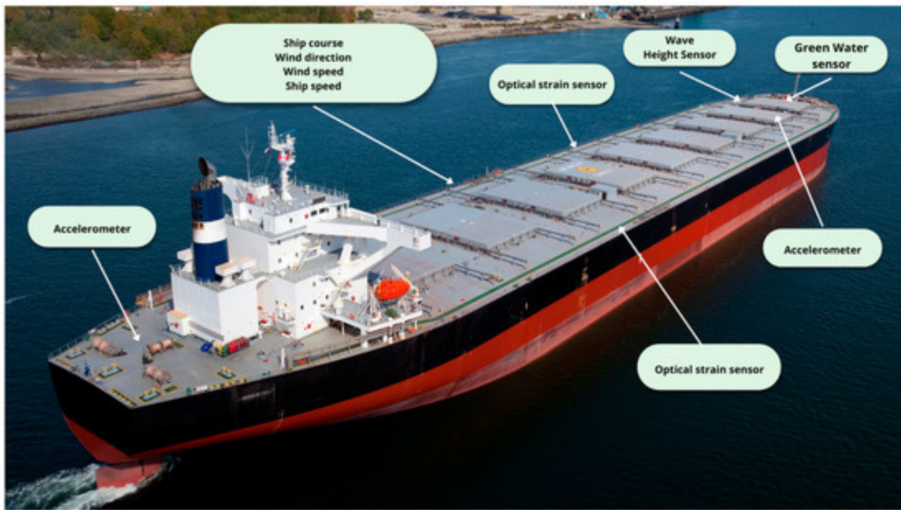
Figure 4 A ship with sensor arrangements [8].
