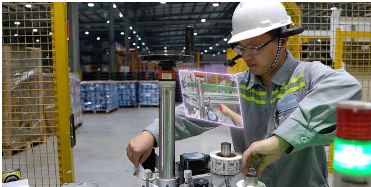
Figure 6 A worker wearing an assisted reality device [12].
