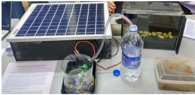
Fig: Experimental Setup of IOT Based Solar Dehydration System with Energy Storage Material for Agricultural products.
