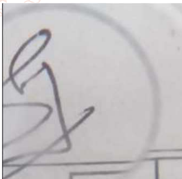
Figure 12 Inkless Starting , Gooping in Glycol based Ink
