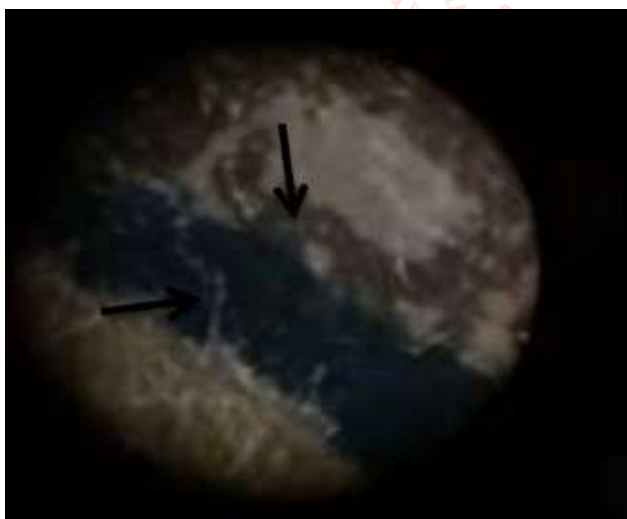
Figure 3 : Scratches from Lead Pencil on Glycol based Ink
