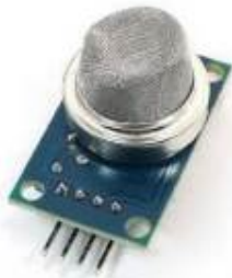
Fig. 2. Gas Concentration: Measured by MQ series sensors (e.g., MQ-2, MQ-135) for sensing LPG, methane, and smoke with readings in parts per million (ppm).
