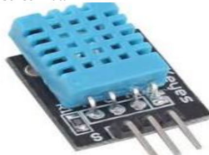
Fig. 1. Temperature and Humidity: Measured by the DHT11 sensor and presented in degrees Celsius (°C) and percentage (%), respectively.
