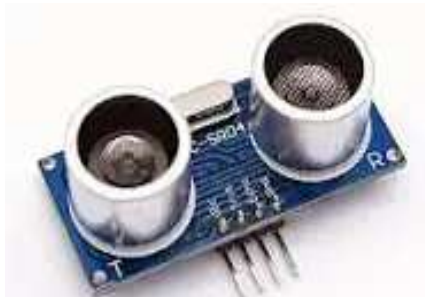
Fig. 3. Distance Measurements: Read using the HC-SR04 ultrasonic sensor, which gives distance measurements in centimeters (cm).
