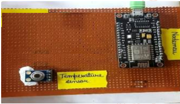
Fig. 8. Project Image with Temperature Sensor and IOT Device.
