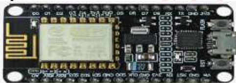
Fig. 4. NODEMCU: Serves as the master microcontroller to read sensor values and send data over Wi-Fi.
