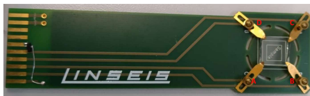
Figure 1. A sample with dimensions of 10×10 mm 2 was mounted in the sample holder.
