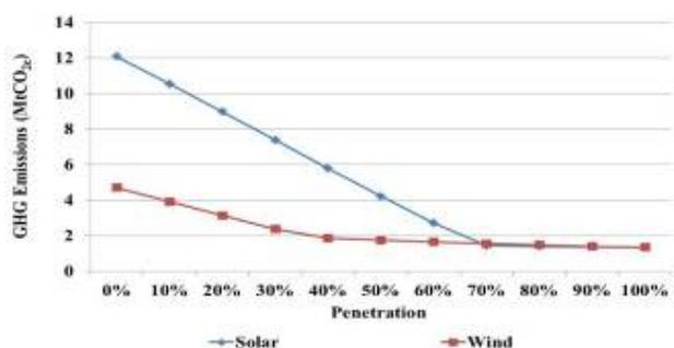
**Fig 10. Variation in GHG emission as solar and wind penetration increases in Myanmar's generation mix**
