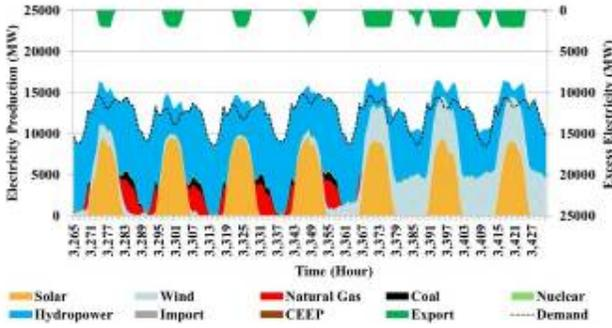
**Fig 7. Hourly data of demand and supply for the RES combination 2030 with interconnection scenario**
