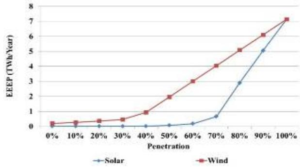
**Fig 8. Variation in EEEP as solar and wind penetration increases in Myanmar's generation mix**
