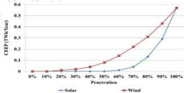
**Fig 9. Variation in CEEP as solar and wind penetration increases in Myanmar's generation mix**
