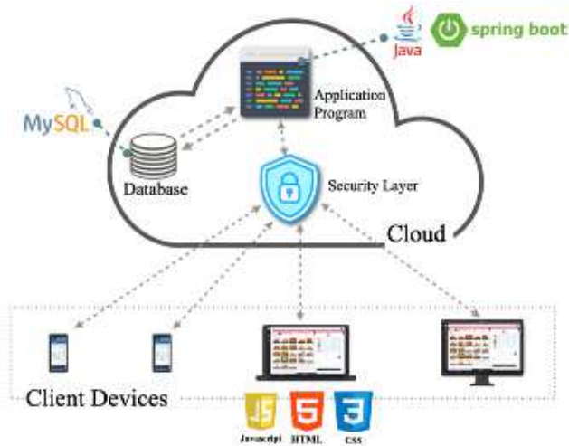
Fig 1: Overall System Architecture
