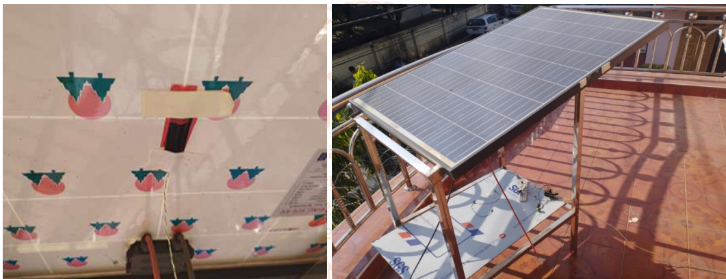
Figure 9. Solar Panel Temperature Measurement System
