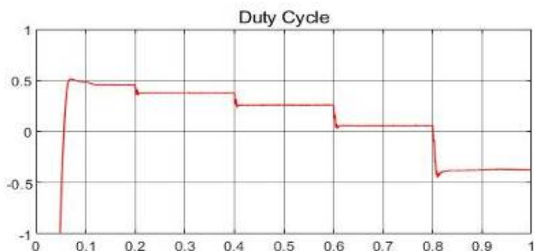
Fig 9 (d): Duty Cycle vs Time in (S) in correspondence with NN – P&O Method.
