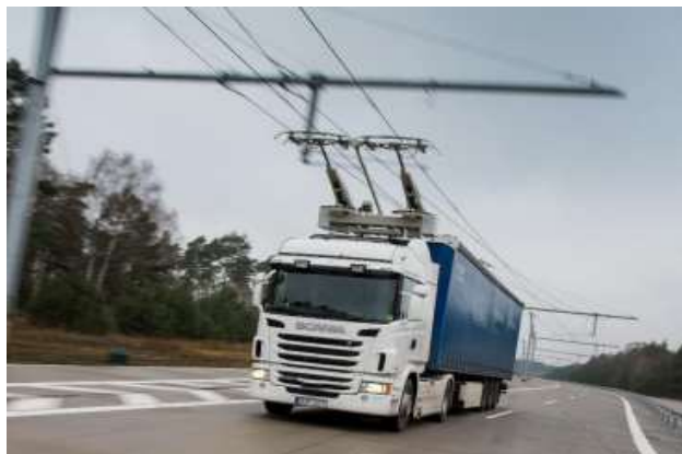
Fig.1. Overhead Conductive Transmission Technology
