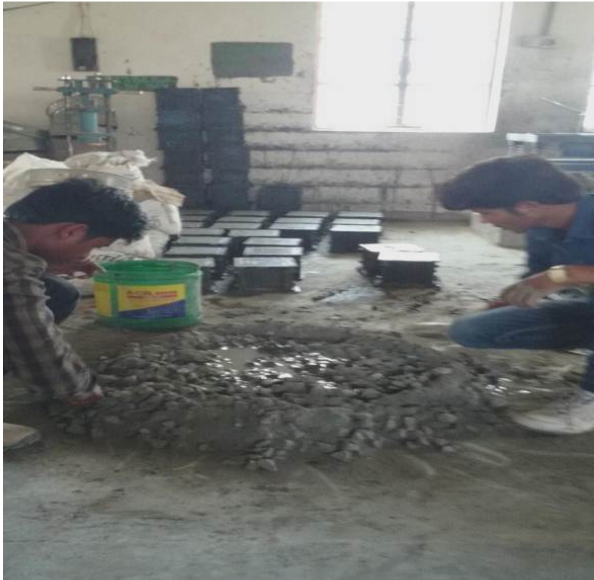
Figure No. 2.1: - MIXING OF MATERIAL M-40
