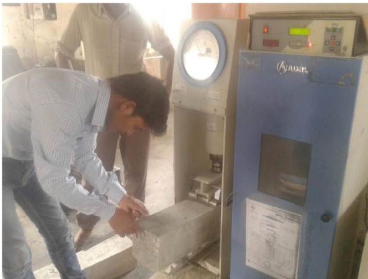
Figure No. 2.7:- FLEXURAL STRENGTH TEST
