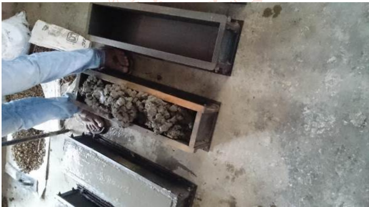
Figure No. 2.2: - BEAM CASTING SIZE 700X150X150
