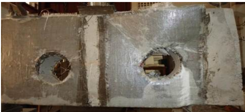
FIG. DEBONDING OF GFRP AT 232 KN
