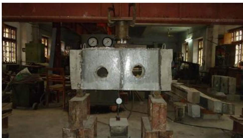
FIG. U-WRAP GFRP WRAPPED AT BEAM 3
