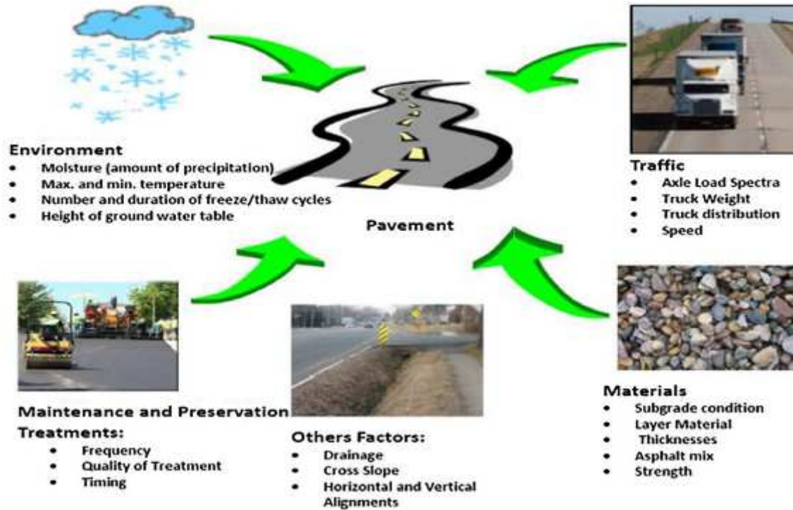
Figure (2): Factors Impacting Pavement Distresses [16].
