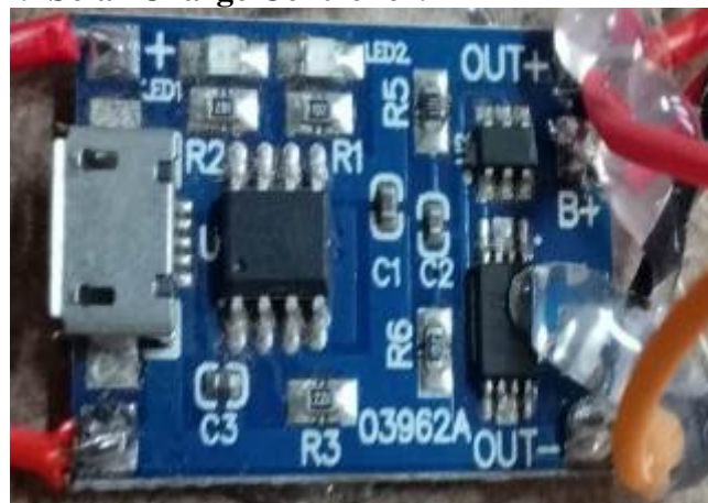
Fig 2; Solar Charge Controller
