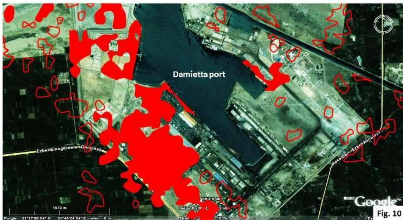
Fig. 10: An enlarged satellite image of the Google Earth program for the port of Damietta on the Mediterranean coast - showing the effect of sea level rise by a maximum of one meter on the facilities built around the port. The completely red areas are the areas threatened by direct intrusion by sea water, while the empty areas marked with red lines are the most important areas threatened by partial immersion in the event of sea water leakage into the subsurface sandy soil.
