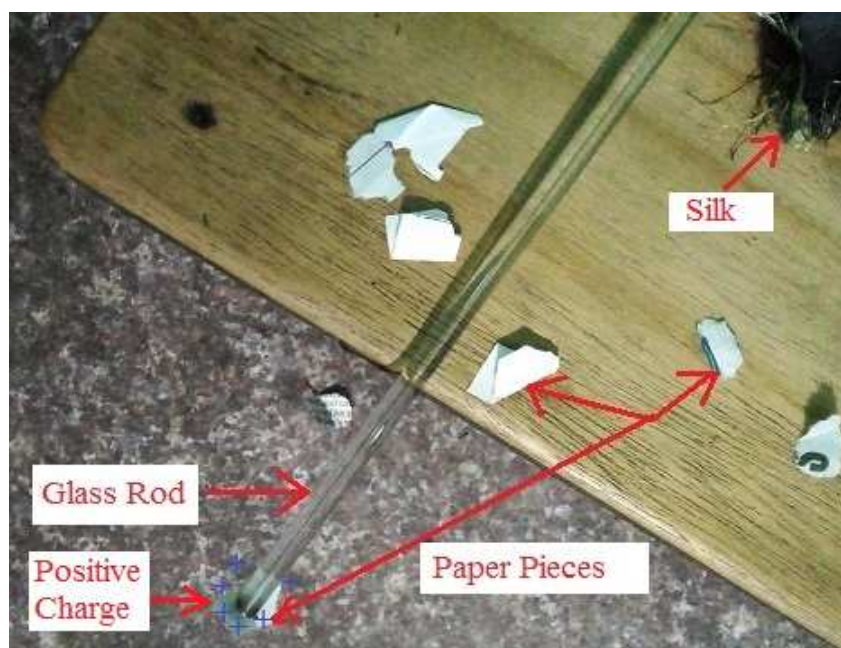
Fig 3 Glass rod rubbed by the silk cloth attracts pieces of paper for different duration of times.
