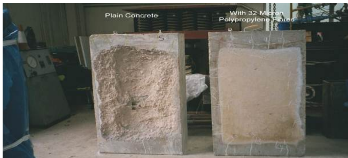
Fig1.2 Comparison of plain concrete with fiber reinforced concrete
