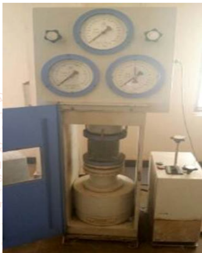
Fig 8.3 Compression Testing Machine with cube specimen
