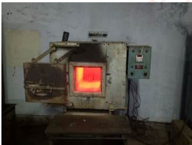
Fig8.2 Annealing gas furnace with burning specimen
