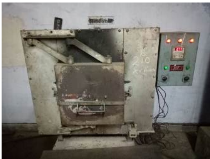
Fig 8.1 Annealing gas furnace
