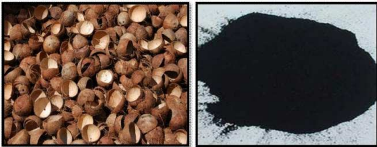
Figure 3. Uncrushed Coconut Shell Sample (a) Crushed Coconut Shell (Ash Form) Sample
