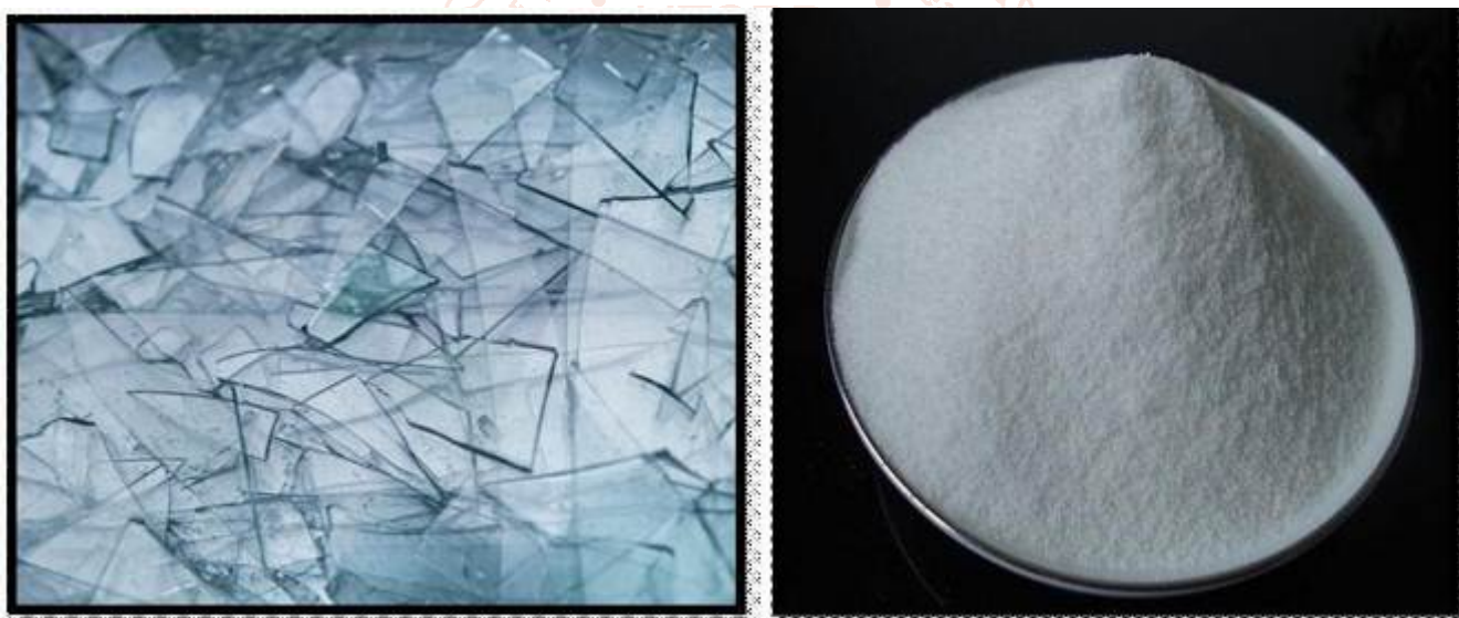
Figure 2 Uncrushed Glass Sample (b) Crushed Glass (Powder) Sample
