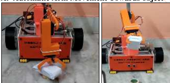
Fig 10 Automatic Arm Movement and Object Lifting
