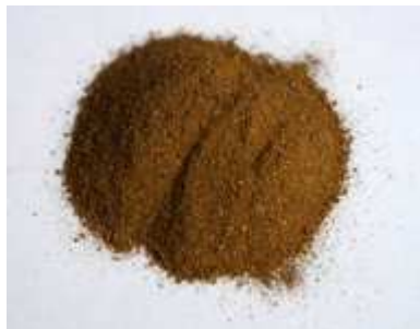
Fig. 4 Titanium Nitride Powder at 0.70 µm
