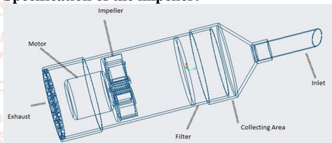
Fig. 1 Components of Vacuum Cleaner
