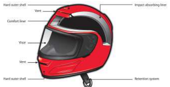
Figure 1. Helmet internal structure (Msf, 2021)
