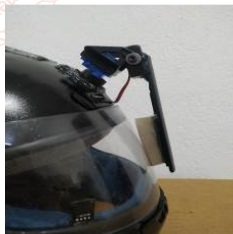
Figure 3. Installation of the wiper system
