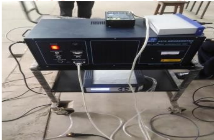
Figure 6 Exhaust gas analyser.
