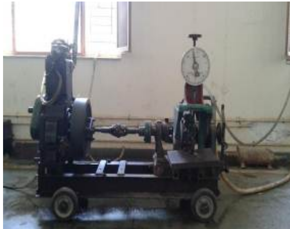
Figure 5. Kirloskar diesel engine with dynamometer.
