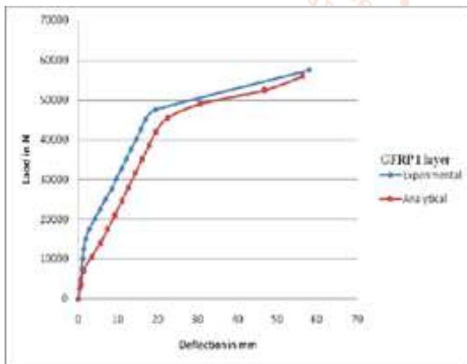
**Fig 7 Experimental and Analytical Load Deflection Curves for Double Layer GFRP Sheet Retrofitted Beam (M 20 Grade)**
