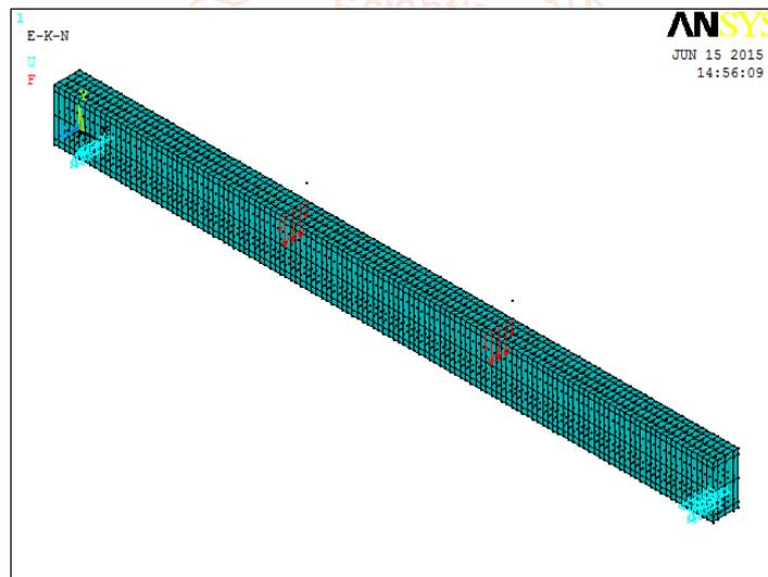
**Figure 4 Loading and Boundary Conditions**
