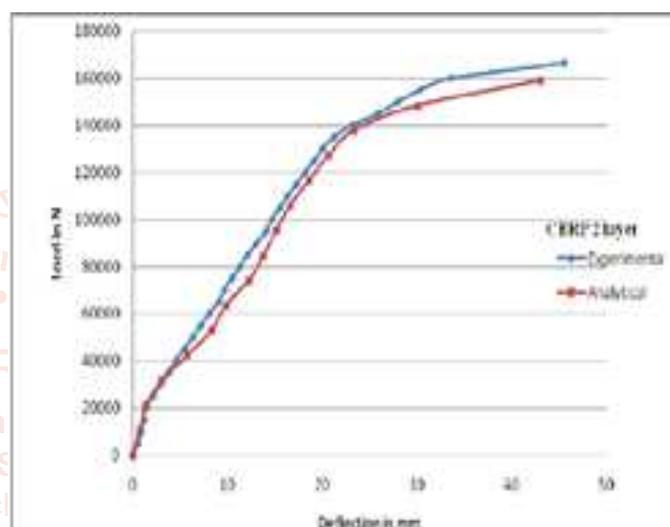
**Fig 15 Experimental and Analytical Load Deflection Curves for Double Layer CFRP Sheet Retrofitted Beam (M 60 Grade)**
