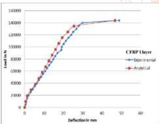
**Fig 14 Experimental and Analytical Load Deflection Curves for Triple Layer CFRP Sheet Retrofitted Beam (M 40 Grade)**
