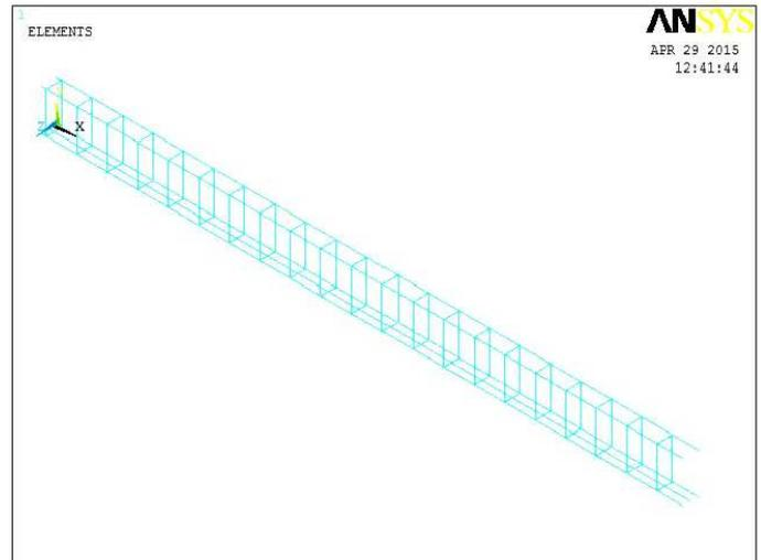
**Figure 3 Meshing of Reinforcement**
