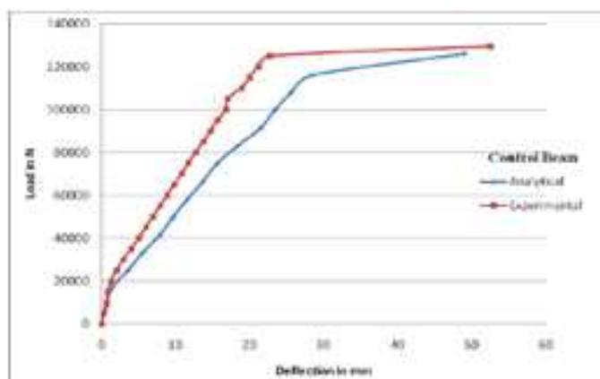
**Fig 13 Experimental and Analytical Load Deflection Curves for Control Beam (M 60 Grade)**
