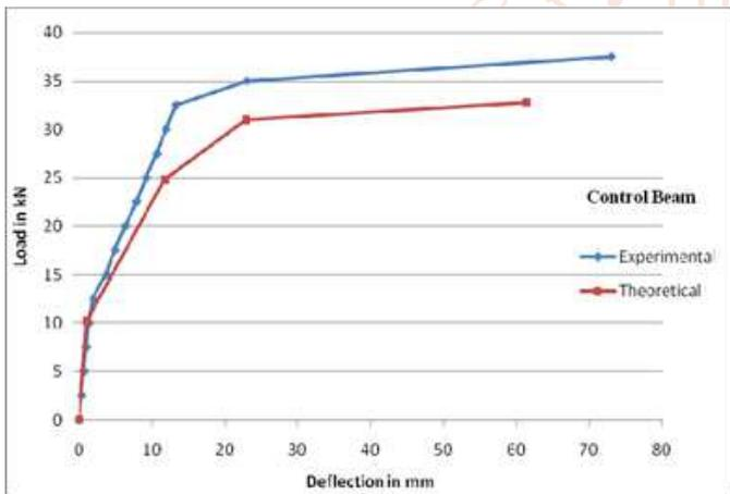
**Figure 17 Experimental and Theoretical Load Deflection Curve of Control Beam (M 20 Grade)**
