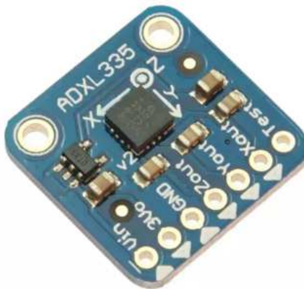
Fig 8. The ADXL335 Accelerometer sensor used in this project for detecting accident along the x, y and z axes
