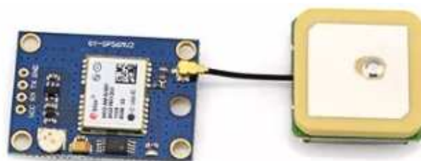
Fig 9. The UBLOX NEO6MV2 GPS module used in this project to send Google Map coordinates of the accident scene
