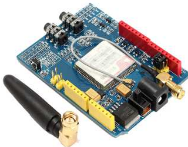
Fig 7. The SIMCOM SIM900 GSM GPRS module for sending CALL/SMS to emergency contact phone numbers
