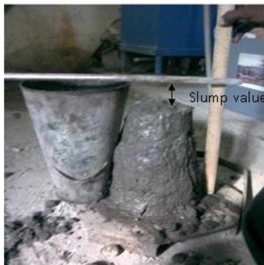
Figure 1. Slump test in progress
