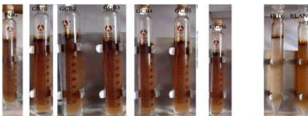
**Figure 17 visual evaluation of 50 ppm dose deoiling efficiency**
