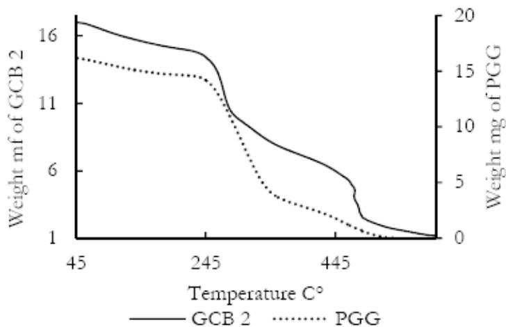
**Figure 7 Thermogram of GCB2**
