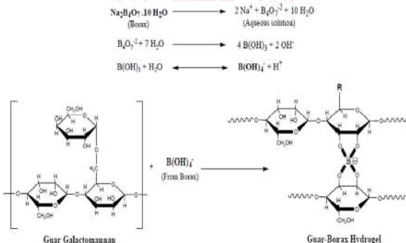
Mechanism of synthesis of borax cross-linked guar gum hydrogels
