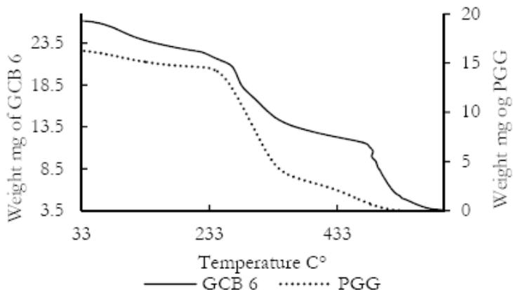
**Figure 11 Thermogram of GCB6**
