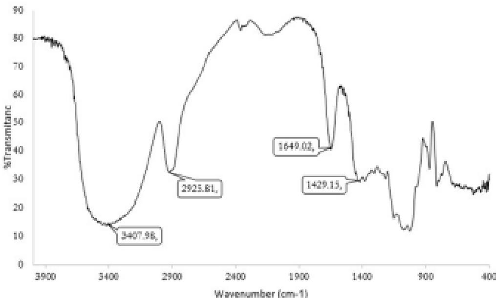
Figure 4 FT- IR spectrum for PGG
