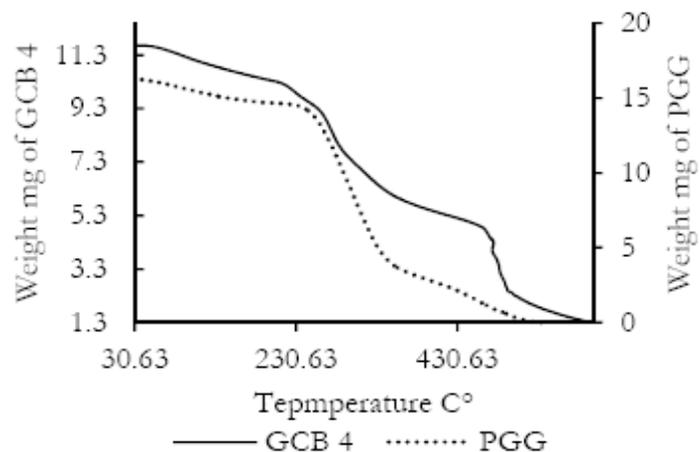
**Figure 9 Thermogram of GCB4**
