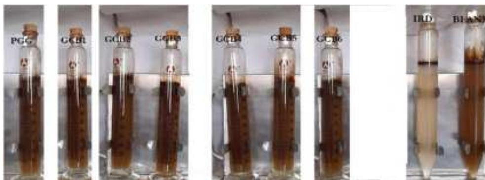
Figure 18 visual evaluation of 100 ppm dose deoiling efficiency
