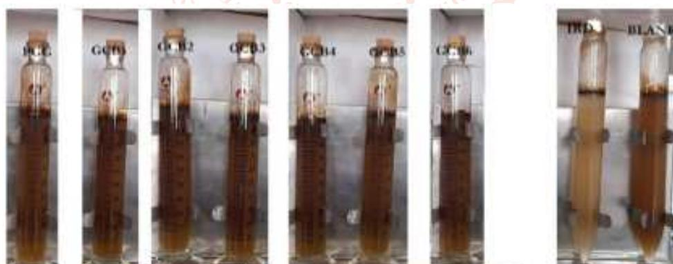
**Figure 16 visual evaluation of 25 ppm dose deoiling efficiency**
