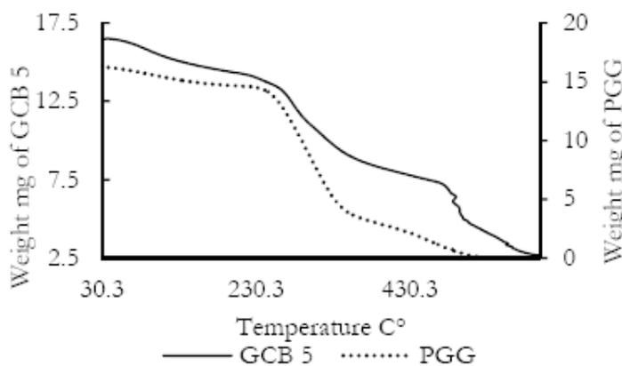
**Figure 10 Thermogram of GCB5**
