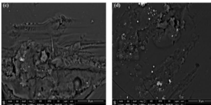
Figure 14 Scanning electron micrographs of GCB (c), GCB4 (d) at (2000x).
