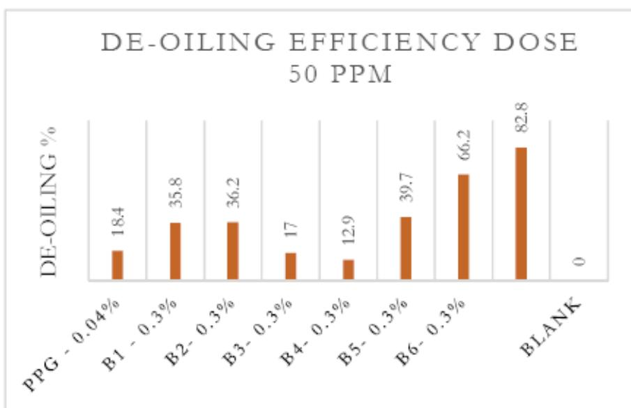
Figure 20 De-oiling efficiency of 50 ppm
