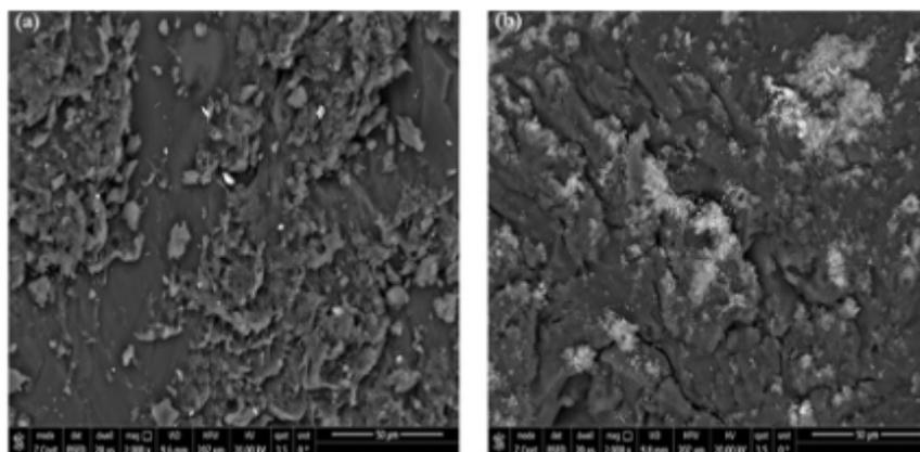
Figure 13 Scanning electron micrographs of purified guar gum (a), GCB2 (b) at (2000x).
