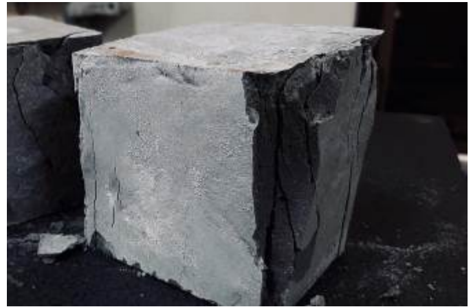
Figure 1. Crushed cement specimen
