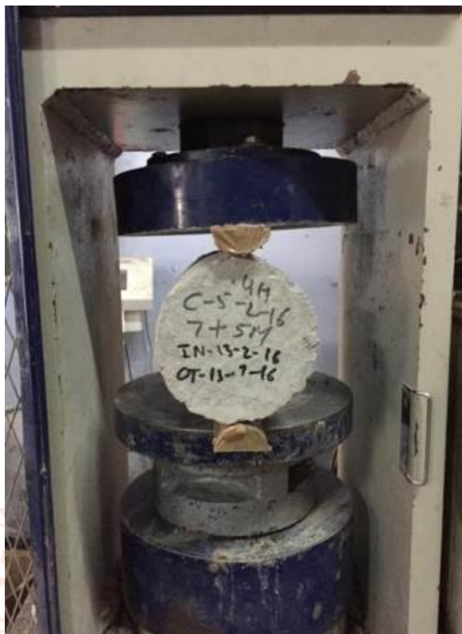
Figure 4.12: Testing of concrete cylinders for split tensile strength
