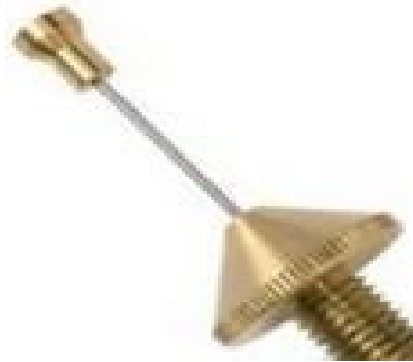
4.9: Needle with annular attachment for Final setting time
