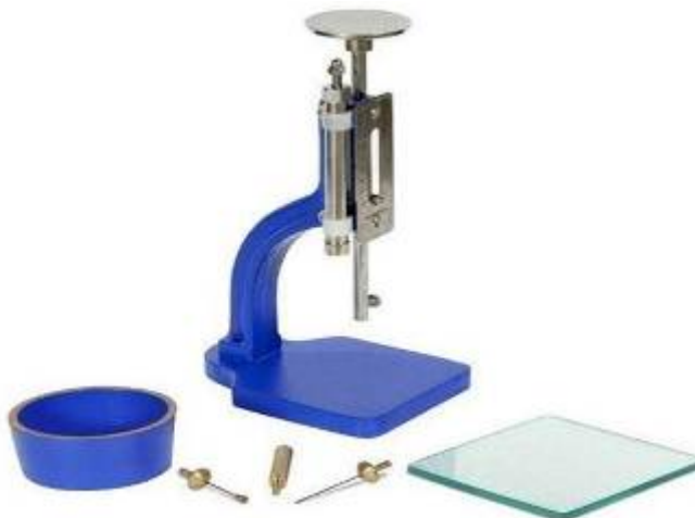
Figure 4.7 : Vicat Apparatus for consistency of cement
