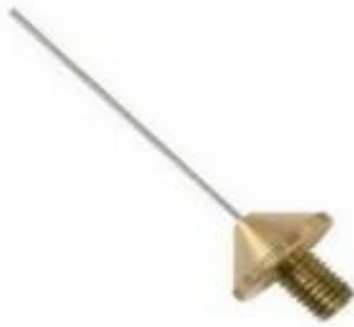
Figure 4.8: Needle used for initial attachment setting time
