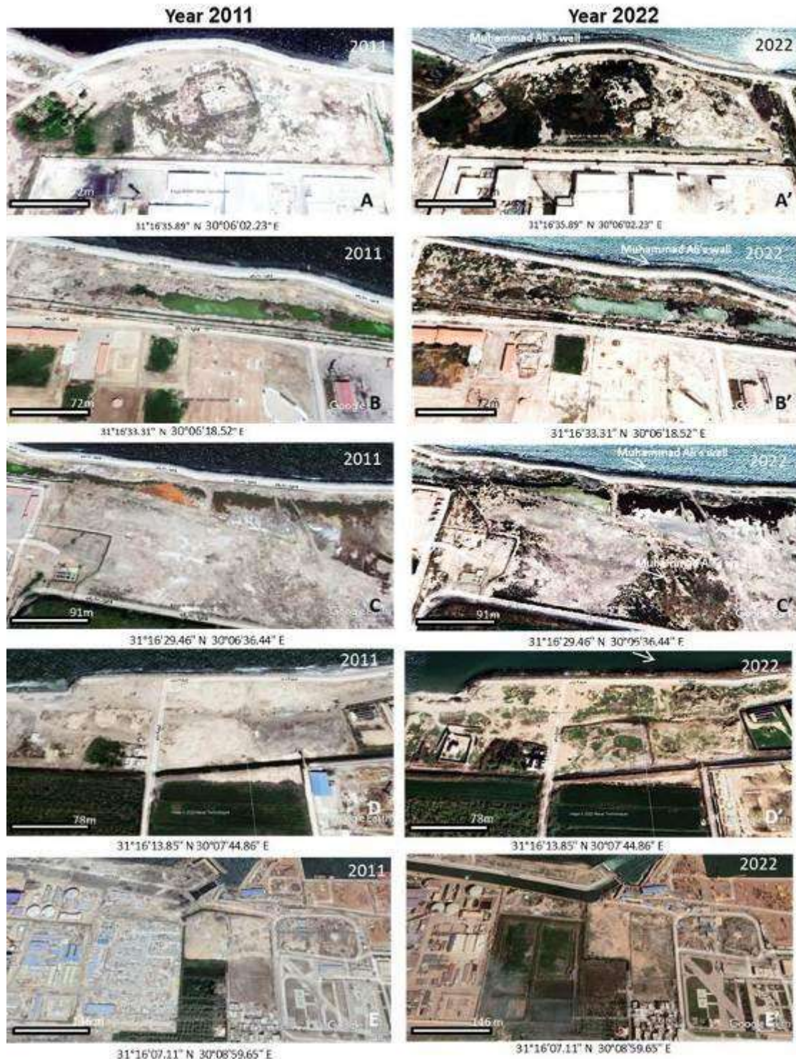
Fig. 10: Satellite images (Google Earth Pro) showing the continuation of seepage of Abu Qir Bay waters into the southern plains along most of the coast during the time interval from year 2011 to year
