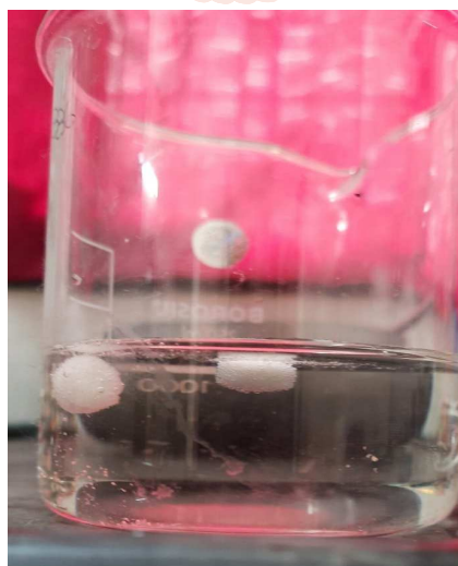
Fig No: 6 in vitro buoyancy study of Metoprolol Succinate floating tablet
