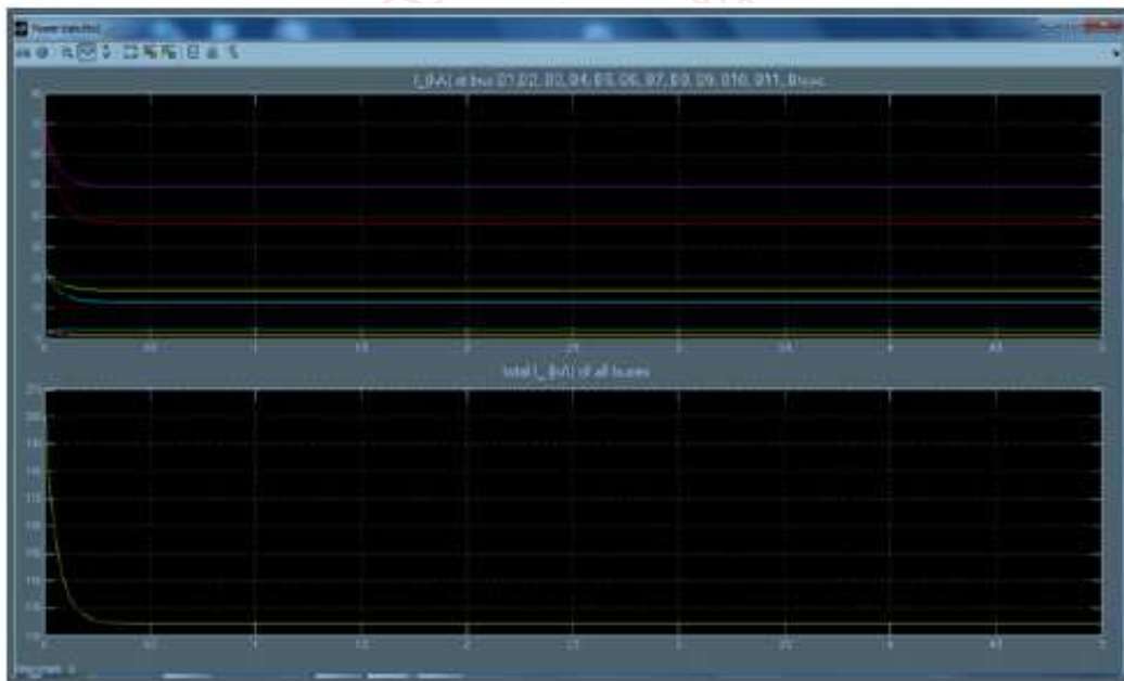
Fig 9 Bus current at different buses and sum of total bus current if SVC connect.
