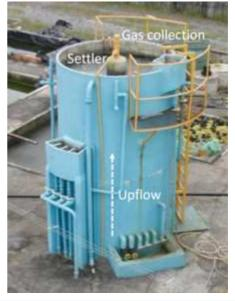
Upflow anaerobic sludge blanket (UASB) reactor
