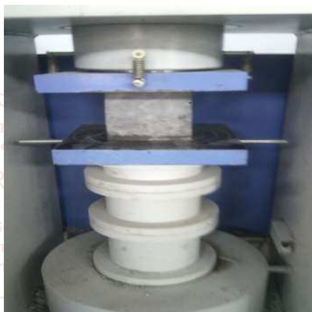
Fig. 1: Test of Concrete for Compressive Strength
