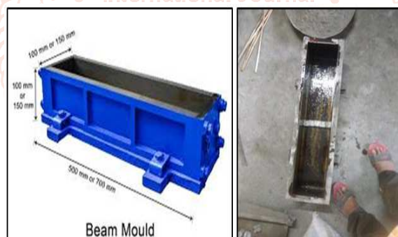
Fig. 2: i) (Left) Standard size of Beam Mould ii) (Right) Mould applied with oil
