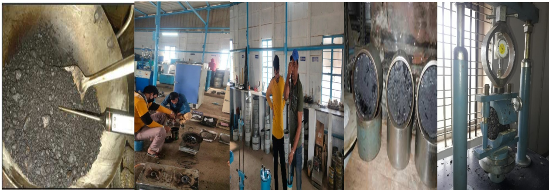
Fig 1.1 Marshall Test being conducted with the Marshall apparatus
