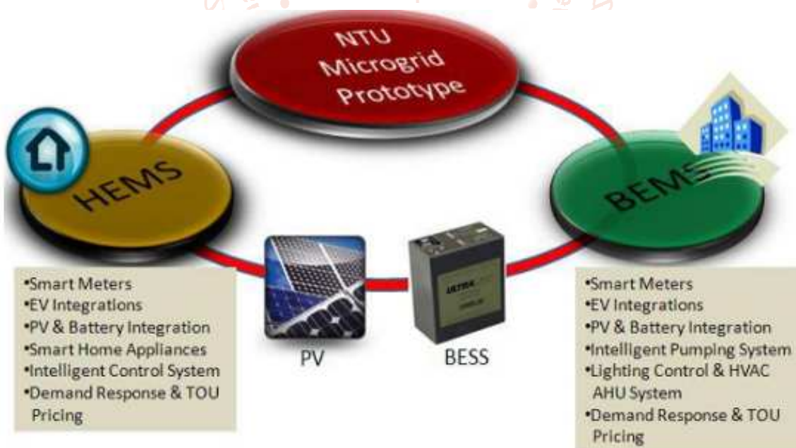
Fig. 3 Smart Grid Architecture
