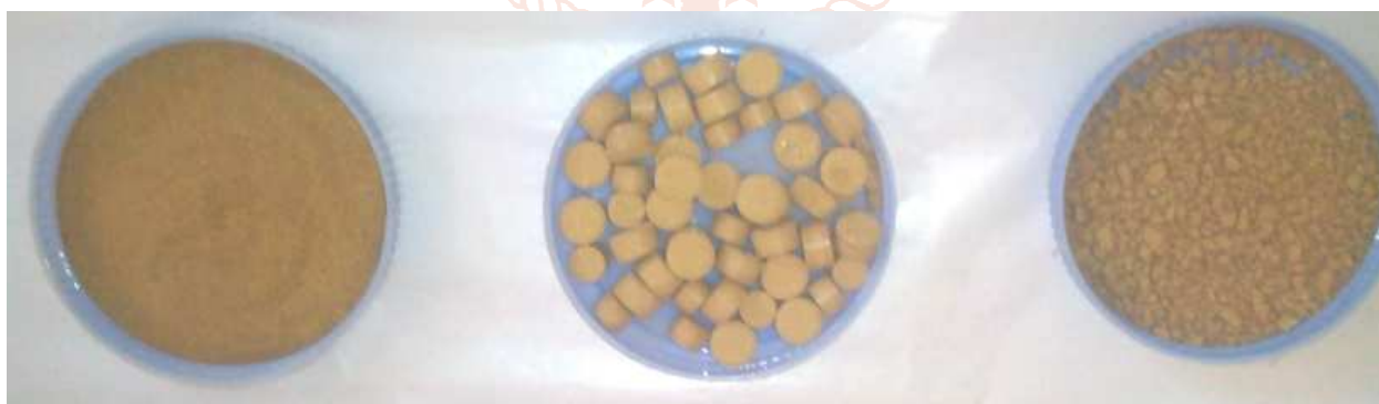
Figure No:-7 Triphala churna powder, slugs and granules (left to right) by dry granulation
