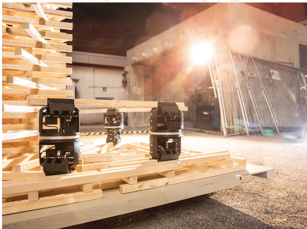
Figure 4 Distributed robotics system for timber construction [15]
