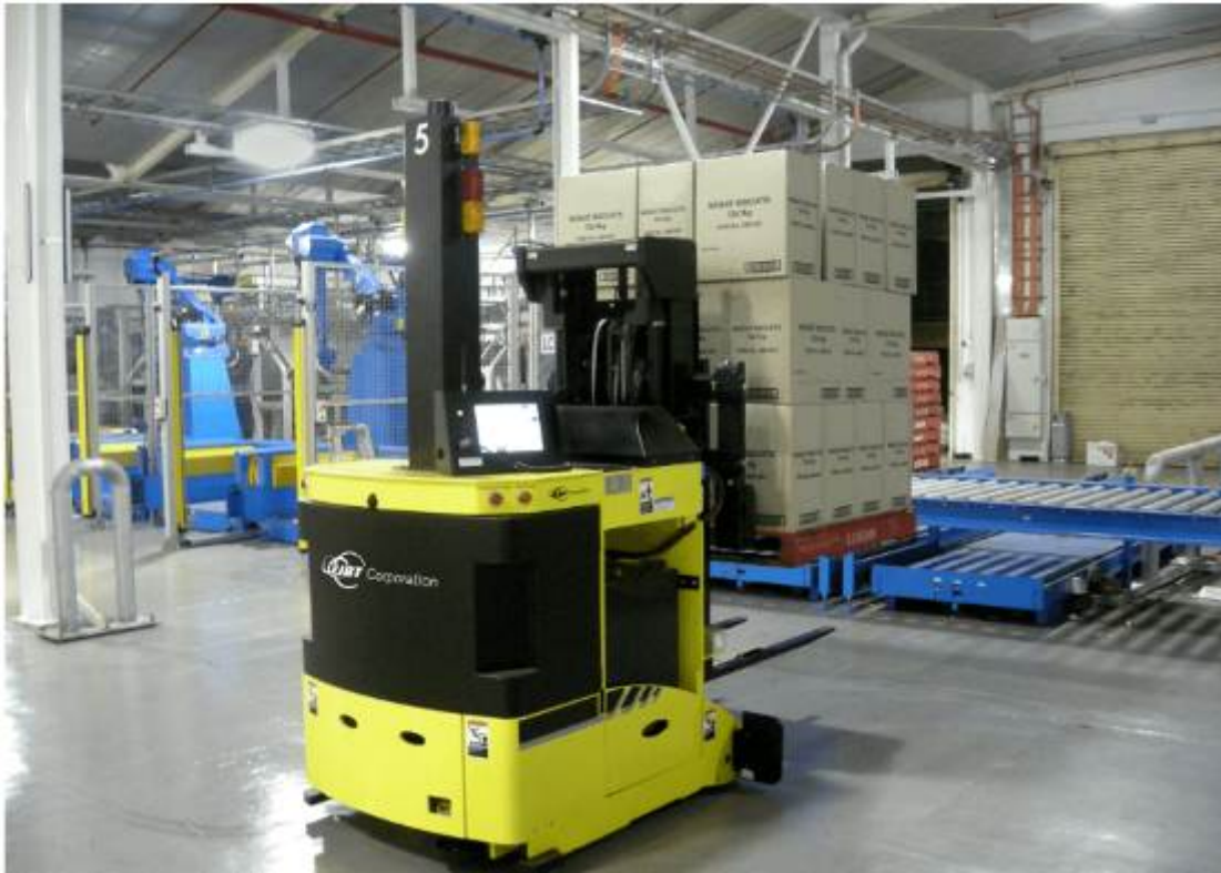
Figure 2 An example of an automatic guided vehicle (AGV) [12].
