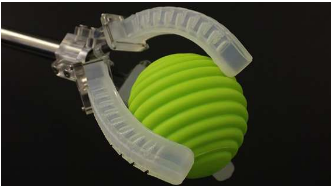
Figure 2 Soft robotic gripper developed using 3D printing [9].
