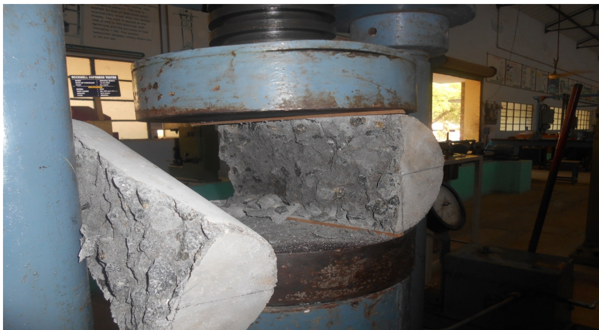
Fig. 3: Testing of cylinder splitting tensile strength of concrete
