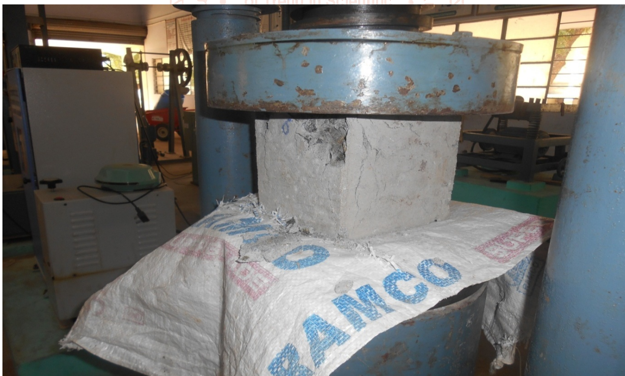
Fig. 1: Testing of cube compressive strength of concrete
