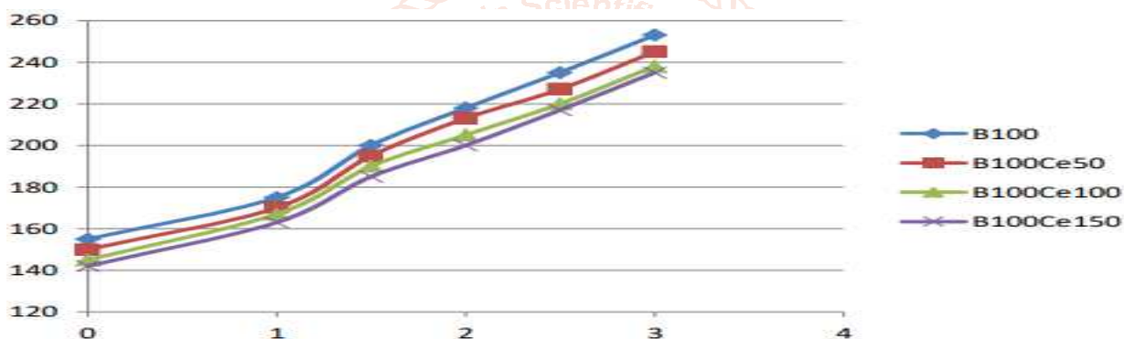
Figure 13 Variation of EGT with load of biodiesel and biodiesel with cerium oxide
