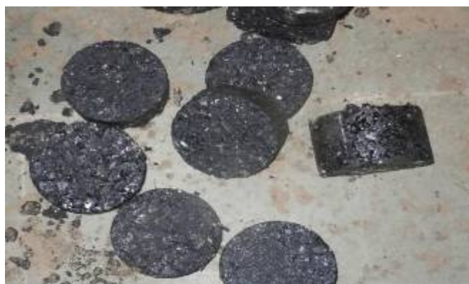
Fig.3.10 SMA mix samples after Marshall Stability Test
