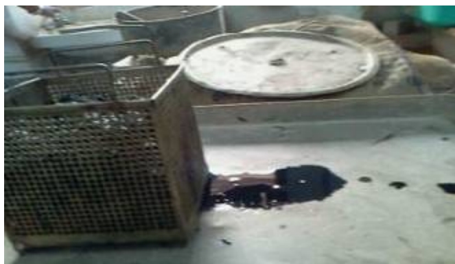
Fig. 3.11 Drainage of 60/70 bitumen sample
