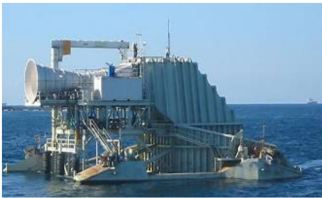
Fig. 4 Oscillating water column
