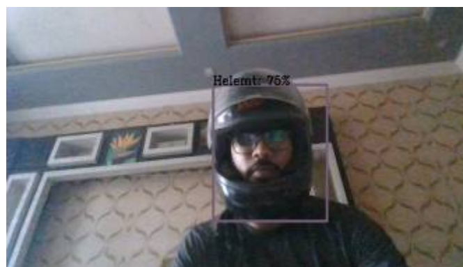
Fig. 4 Helmet is detected with a probability of 75%
