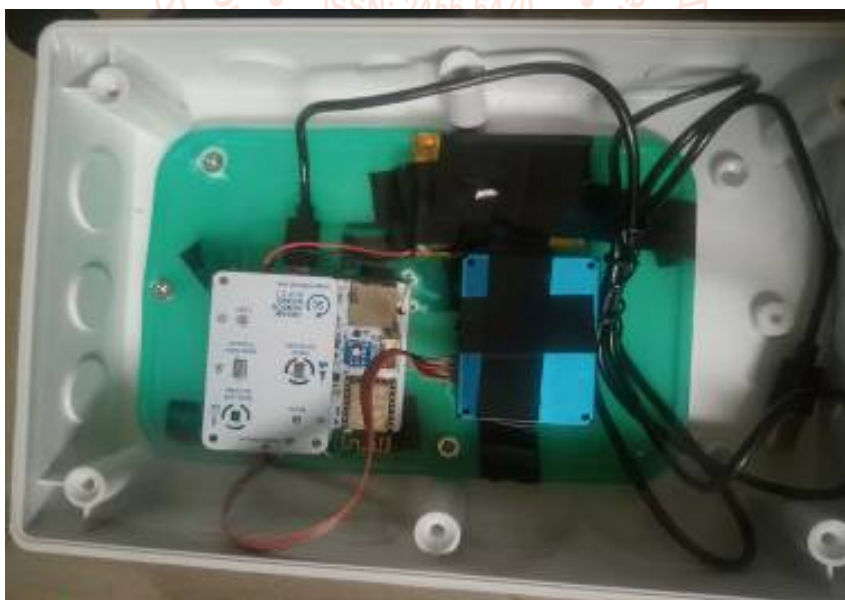
Fig 3 The Air and Sound Pollution Monitoring System packaged in a IP66 enclosure
