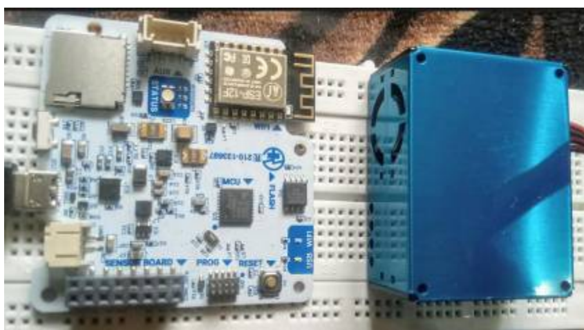
Fig 2 The Urban Sensor Board and Particulate matter sensor (PMS 5003) on breadboard
